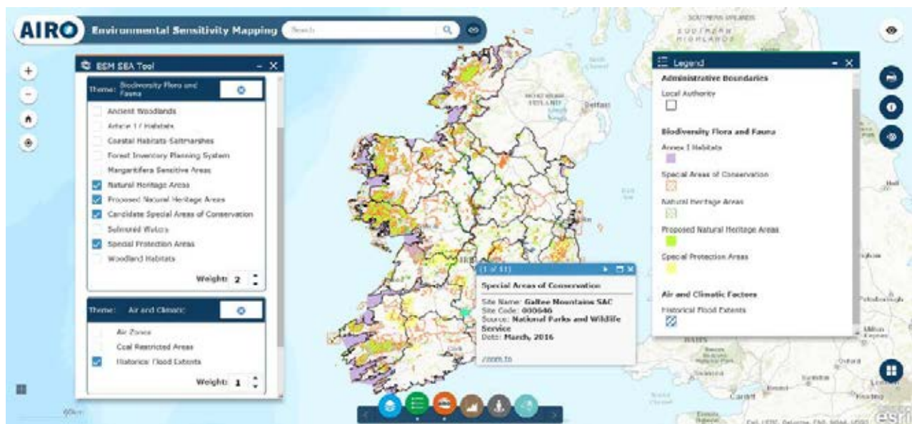
Figure 5.1. The ESM webtool interface illustrating the spatial datasets available in the viewer (right), the query tool (centre) and the widget (left), where themes/criteria and weights can be defined for their combined assessment.
